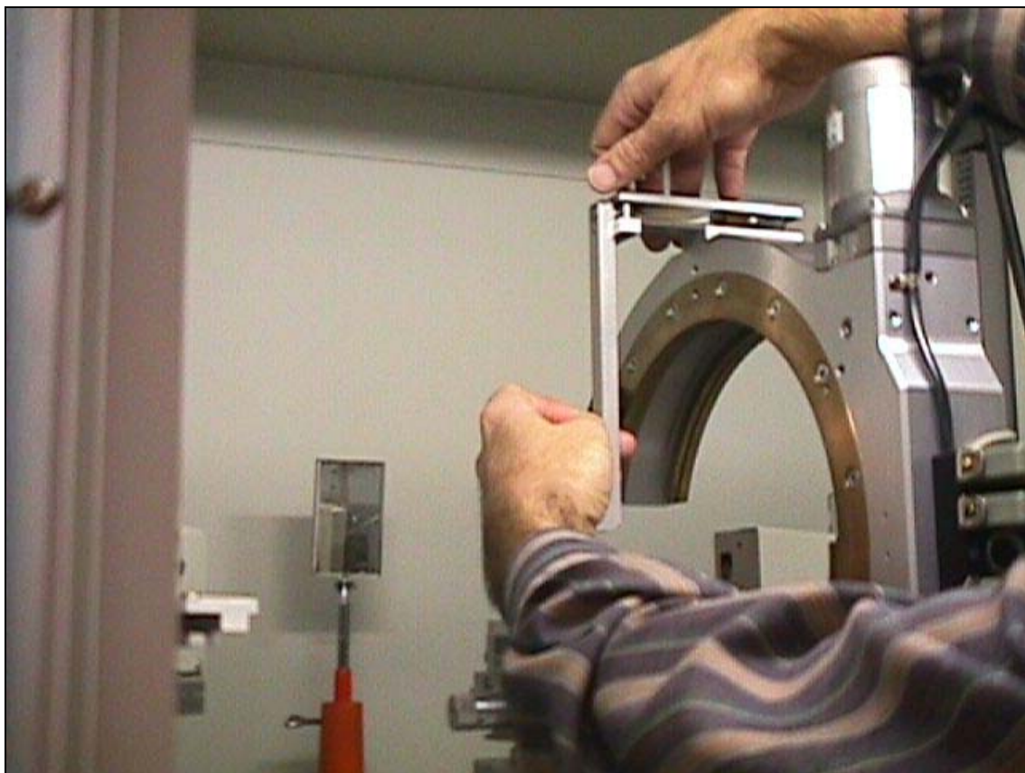
9.3.4 Next, take the dial indicator in your right hand by the mounting arm.
