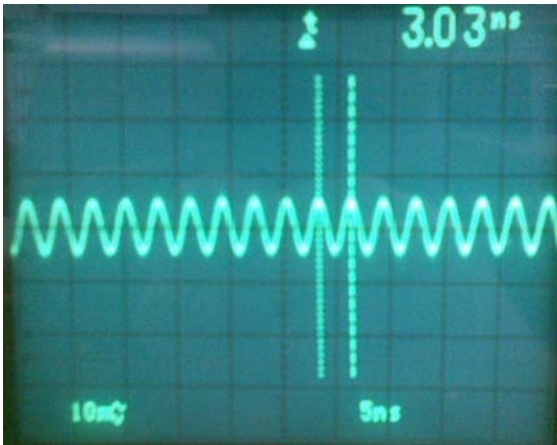
Figure 6 - One of the Faster Ring Oscillators on the Test Chip (W = 2.5 μm and L = 0.3 μm)
