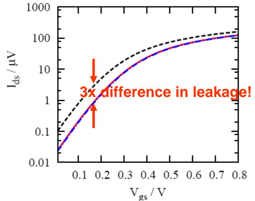
NMOS Leakage with  $V_{ds} = 1.2V$
