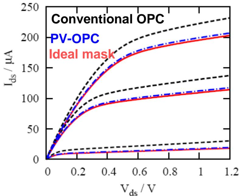
I-V curves with  $V_{gs} = 0.4, 0.8, 1.2V$
