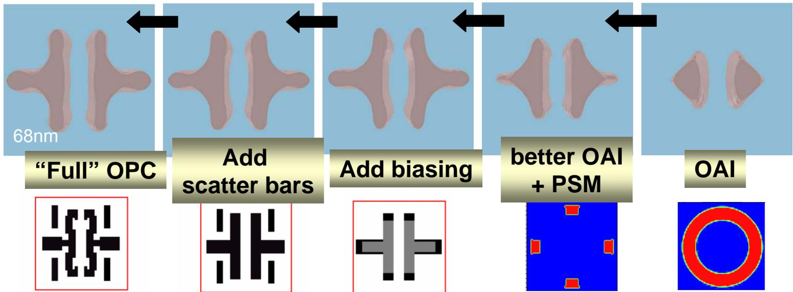
**OPC: optical proximity correction; OAI: Off-axis illumination** (Source: ASML)
