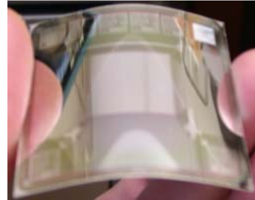
steel foil substrate
