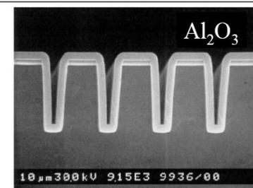
Precise film thickness control by the number of deposition cycles
