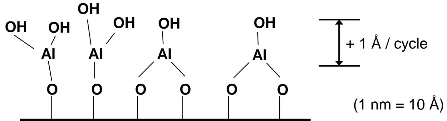
100 cycles → 10 nm      1000 cycles → 100 nm
