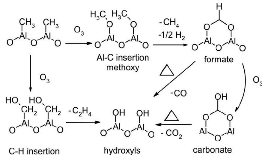
**Figure 14.** Proposed mechanism for O<sub>3</sub> reaction during Al<sub>2</sub>O<sub>3</sub> ALD using TMA and O<sub>3</sub>.
