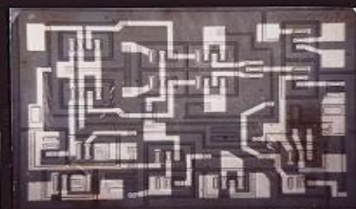
Low-Distortion Wide-Band Variable-Gain Amplifier W. Sansen, Prof Meyer 1972
