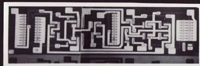
Drift/Offset Compensated Amplifier G.L. Baldwin, Prof. Pederson 1969
