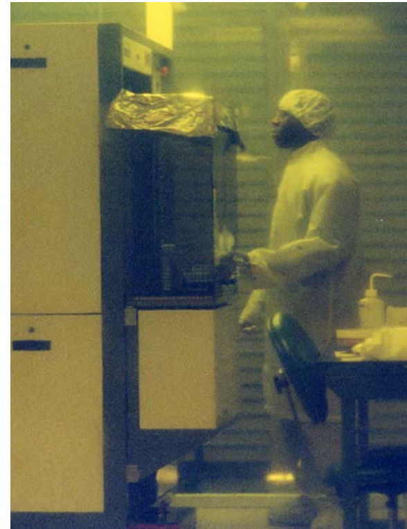
Alcatel 601-E etcher >1 million microneedle chips annually
